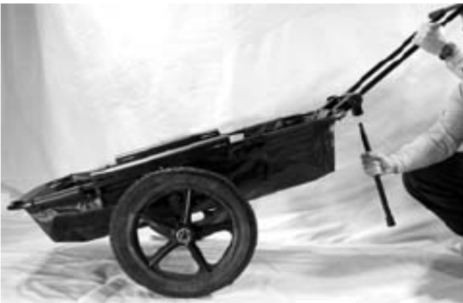
8. Place Kickstand into female receiver located at bottom of handle. (Note: Remove Kickstand once unit is loaded and store in horizontal storage hole located in female receiver prior to moving forward).
