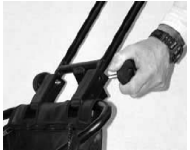
7. Place unit onto its wheels and insert handle (Note: You must remove stainless steel studs from female receivers before inserting Handle). Replace stainless steel studs and secure
