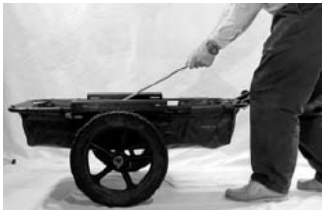
9. Insert Hard Polymer Bottom into unit.
