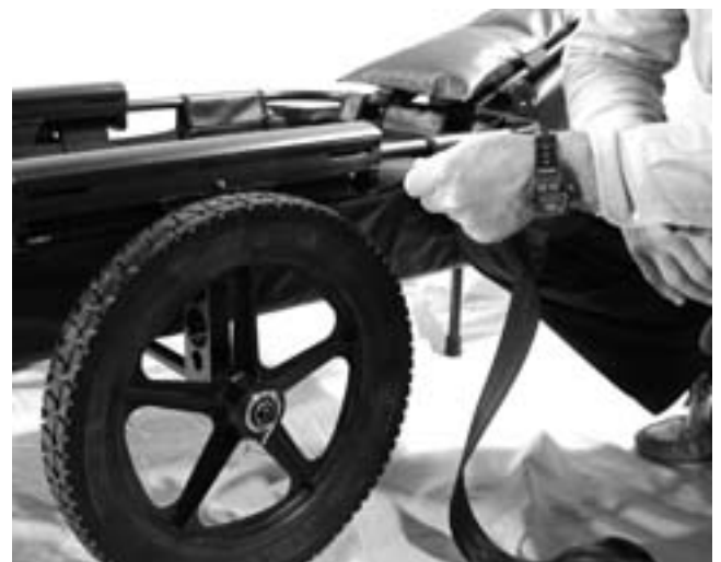
18. If straps are required to secure load, insert them through slots located at either end of the rails as shown.
