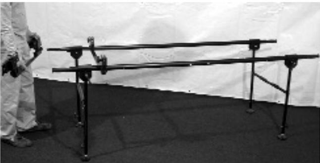
28. Take the Stretcher Clamp Assembly which has the Stirrup IV Blocks and slide onto the Support Tube Assemblies making sure ratchet handles are facing outward.
