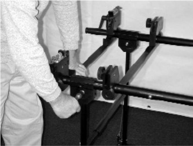
35. Once Leg Supports have been tightened, secure Leg Assemblies to 1 1/2" Support Tube Assemblies. Secure all four clamps.
