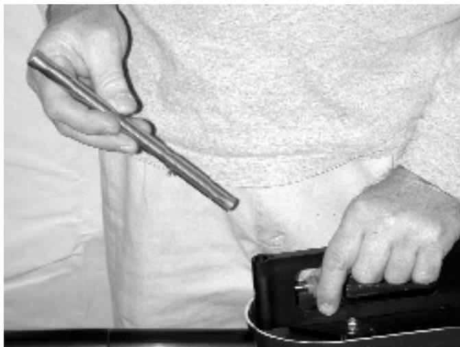
49. Remove the short 1/2" stainless steel shaft packaged with the Arm Boards and insert them into the bottom receivers as shown (**NOTE: It is necessary to loosen the Red button prior to insertion; retighten once complete**). Now insert the Arm Boards into the Accessory Clamps previously installed and tighten as shown above.
