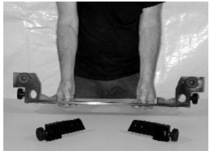
20. Remove the Stirrup Crossmember (1) and Stirrup Keys (2) as shown above.
