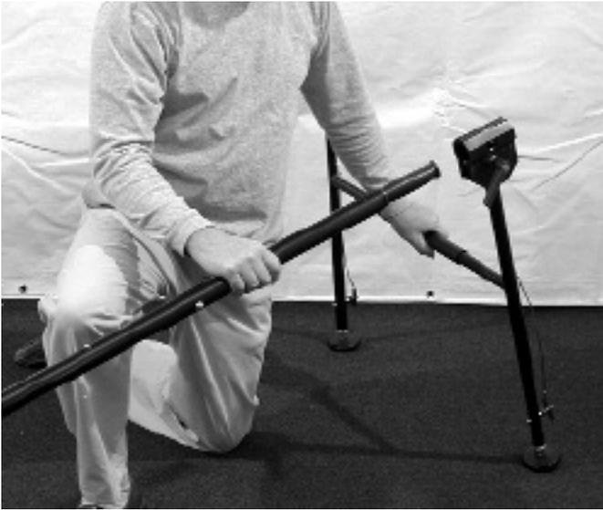
17. Place one Support Tube Assembly through the hole located at the top of the Leg Assembly making sure 5/8" Snap Buttons face outward. Allow the Support Tube to extend beyond the Leg Assembly approximately 6". Do not secure at this time
