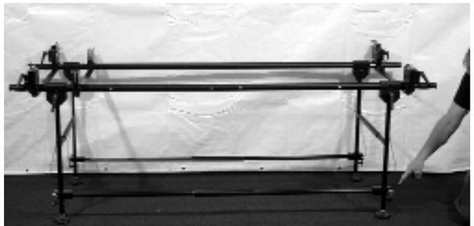
34. Secure Leg Support to Legs as shown. Clamp to leg above T-Pin. Repeat this procedure on all four legs. Secure Leg Supports but do not tighten down at this time. **NOTE: Before proceeding to tighten Leg Supports check to make sure table is square. Now tighten Leg Supports to Leg Assemblies.**
