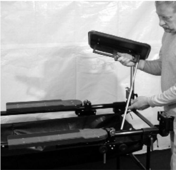
51. Mayo Tray is installed the same as the Arm Boards. The only difference is the length of the 1/2" stainless steel shaft. The Mayo Tray is usually located at the head utilizing the same Accessory Clamp as one of the Arm Boards **(NOTE: The Mayo Tray can be placed along the entire Support Tube Assembly).**
