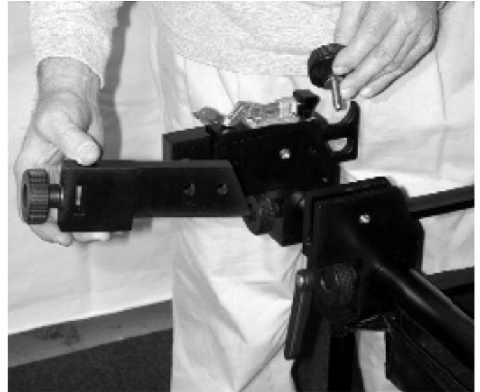
42. Remove the Stirrup Keys from Accessory Kit B (Stirrups). Remove the 2" threaded knob from the Stirrup Crossmember and insert the Stirrup key into the Crossmember as shown. Replace 2" threaded knob (**NOTE: Do not fully tightened at this time**).
