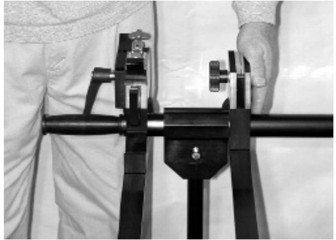
36. Slide Strirrup Crossmember up against the Leg Clamp as shown and secure both sides.
