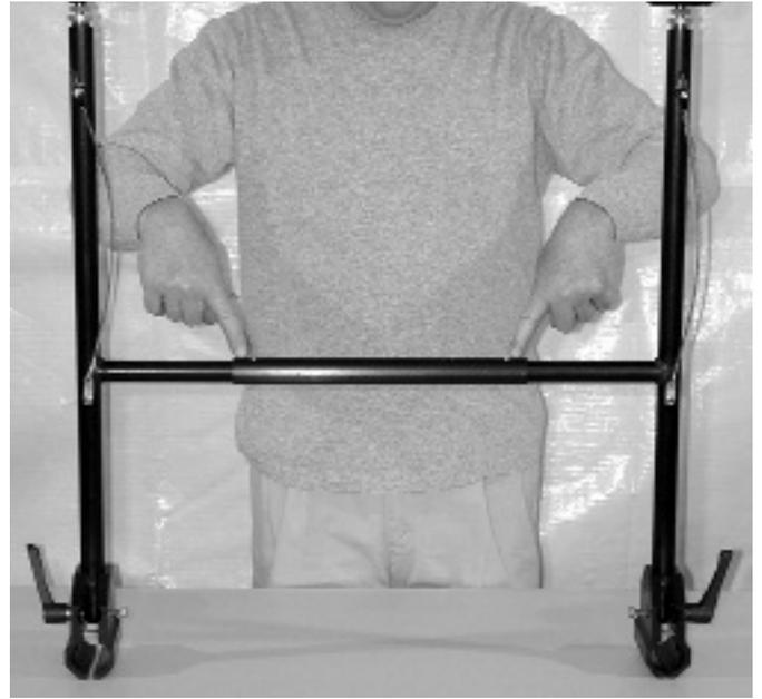
15. Begin by depressing the 1/4" snap button and sliding the legs to the outermost holes.
