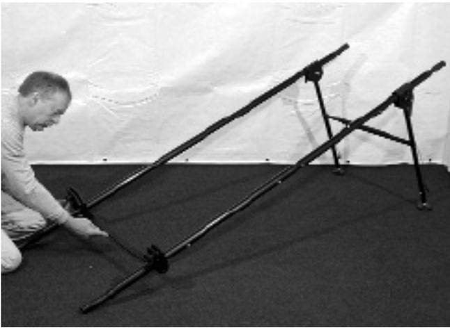
26. Take Stirrup Crossmember (Photo 20) and slide onto the ends of Support Tube Assemblies. Position approximately 12" as shown and secure by tightening the 2" knob located on the side of the Stirrup Crossmember.
