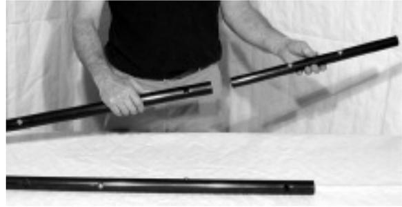
6. Insert the connector tube into one of the long support tubes as shown until the large snap button engages the corresponding hole.
