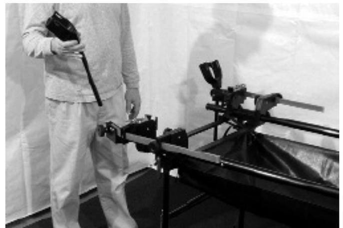
44. Picture above shows proper installation of Stirrup Rail. It is now time to insert Stirrup into Stirrup Rail as shown. (**NOTE: By reversing Stirrup Rails from one side to the other the spread is increased or decreased by 6"**).
