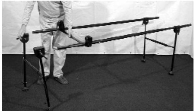
27. Holding the Stirrup Crossmember as shown, slide the remaining Leg Assembly onto the Support Tube Assemblies making sure that the T-Pins (Photo 16) are facing outward. Again, Allow the Support Tube Assemblies to extend approximately 6" beyond the Leg Assembly.
