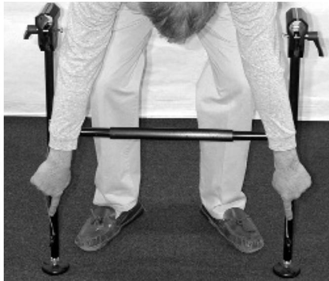
16. The preassembly is complete and now we are ready to begin the assembly of the SR901RT. Make sure the T-Pins at the bottom of the legs face outward during set-up.
