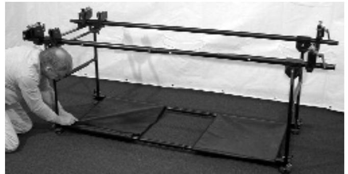
37. Remove Mesh Shelving (2), fiberglass Lower Shelf, Leg Support Crossmembers (2) and Fluid Capture from level three in Carry Bag. Begin by wrapping the Mesh Shelf around Leg Supports and close zipper. **NOTE: It is much easier to accomplish this if you zip from the inside towards the outside.** Once zipper has been secured rotate zipper until it is underneath shelf. Repeat this procedure at the other end of the table.
