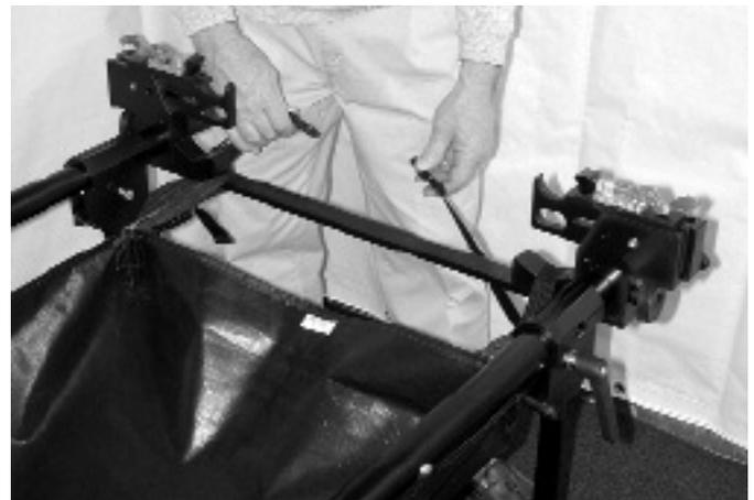
40. With the four short straps attached it is now time to secure the four long straps. This is done by passing these straps around the Legs as shown above and secure (**NOTE: Do not tighten at this time**).
