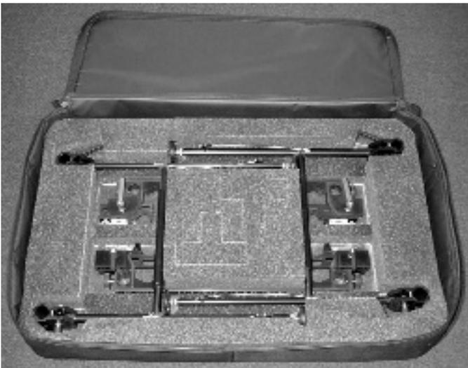
3. Level two includes the Legs and Stretcher Clamp Assemblies.
