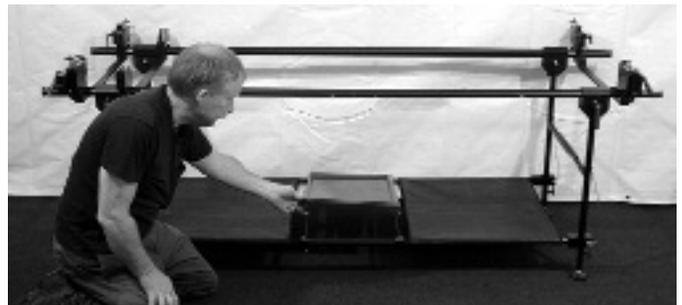
38. Drop both Leg Support Crossmembers over Leg Supports on either side of connector tube and place fiberglass Lower Shelf over Leg Support Crossmembers.
