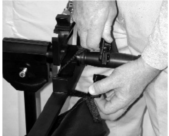
39. To install Fluid Capture, roll out as shown above making sure high gloss side is facing up. Note there are four short straps located in each of the four corners along with four longer straps. Disregard the four longer straps for the time being. Begin by securing each of the four short straps over the V-block located on each Stretcher Crossmember (**NOTE: It may be necessary to loosen these straps to attach all four, they will be tightened later**).
