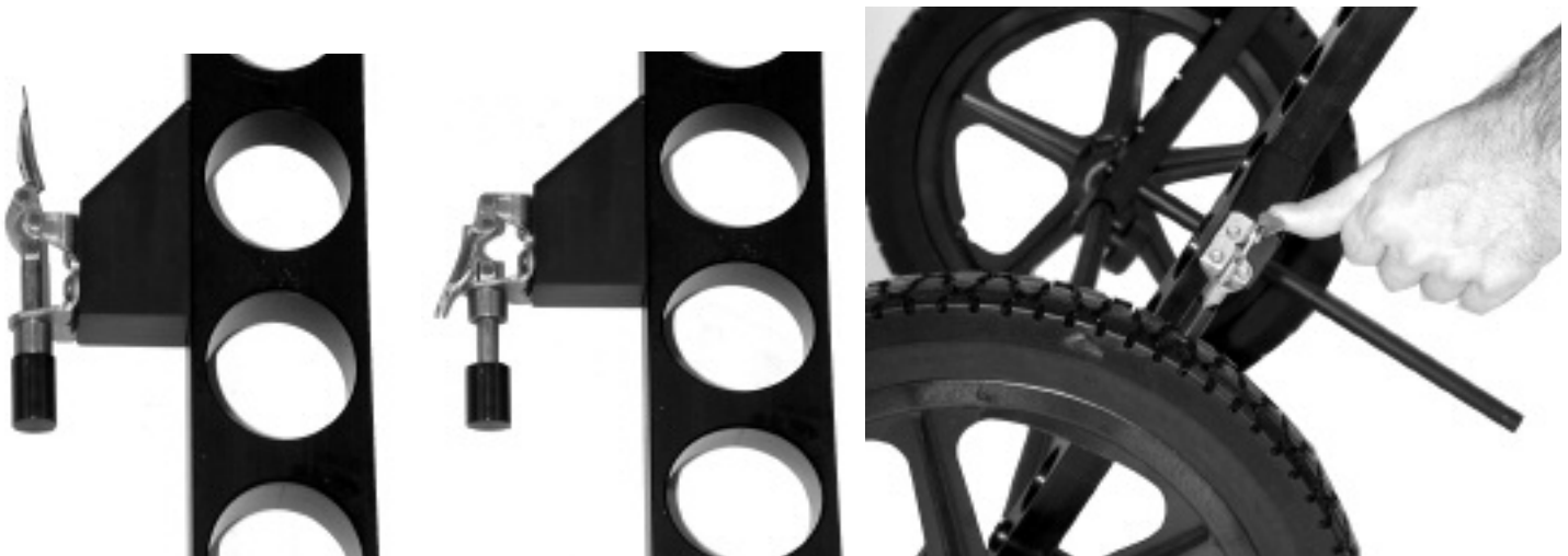
18. SR801RT Brake detail. To activate Break press down as illustrated above.
