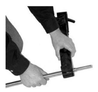
3. Slide the stainless steel Axle through the 3/4" hole located at the bottom of the 7 hole Stanchion to the inner most groove located on the Axle. Secure Axle in place by tightening knob located at bottom of Stanchion. Repeat procedure for the opposite Stanchion.
