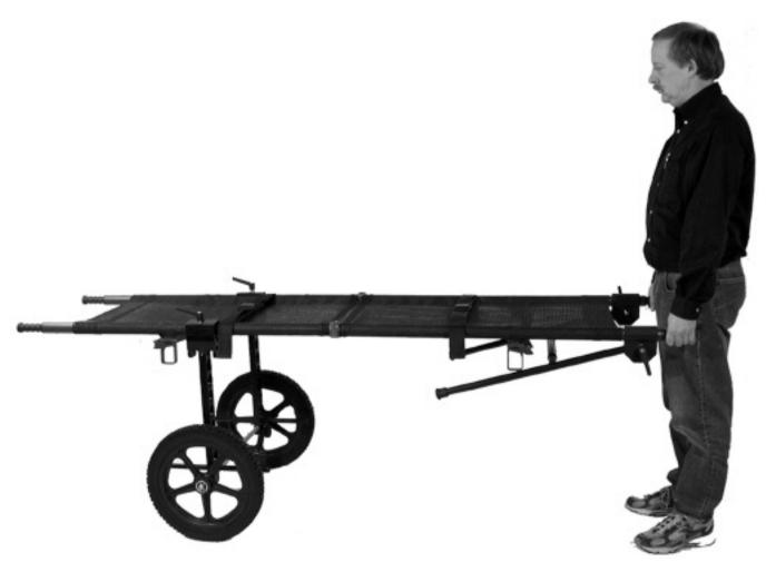
11. Kickstand can be folded up and out of the way when it is necessary to travel over uneven terrain or long distances. This is achieved by loosening the Kickstand clamp until legs fold up and then retighten clamp. NOTE: It is not necessary to fold Kickstand to transport injured.
