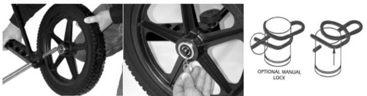
6. Install Wheels and insert Rue pins to secure. To install Rue Pins push into hole at end of Axle and they will snap secure. To lock Rue Pins in place activate optional manual lock. To remove Rue Pins unlock and lift end of pin which has slight bend and pull.(NOTE: Rue Pins are stored in pouch.)
