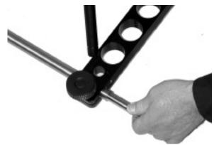
5. Slide 16" Kickstand into 3/4" hole located directly above Axle as illustrated. NOTE: There is a groove located at either end of the Kickstand, this will be engaged by a stainless steel ball plunger located within Stanchion.
