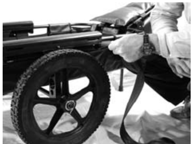
18. If straps are required to secure load, insert them through slots located at either end of the rails as shown.
