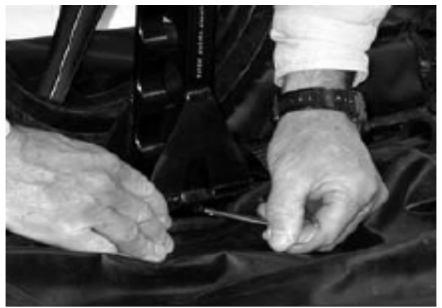
6. Insert Release Pins as shown.
