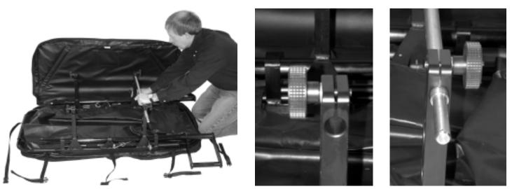
6. Loosen axle clamps (close up) and slide axles into place. Twisting axles into place prevents "jacking". Secure Axles by tightening axles clamps when axle grooves match outside stanchion edge and hole in end of axle faces up. (see close up of axle clamp and axle).
