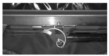
14. Insert locking pin with handle in upright position. Repeat for the other handle (slide out, rotate and insert pin).
