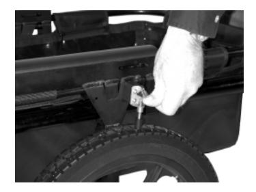
15. Apply brake by pressing lever handle on brake assembly until it locks down. To release brake pull up on brake lever.
