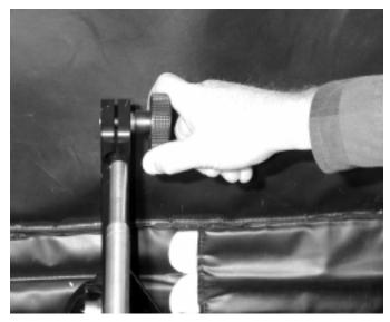
5. Loosen axle clamps (close up) and slide axle into place. Twisting the axle into place prevents "jacking". -Secure Axle by tightening axle clamps when outer most axle grooves match outside the stanchion edge. Note: the hole in end of axle faces up.
