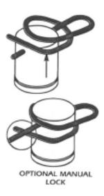
6. Remove Rue Pins (Axle Pins) from pouch on top of canvas carry case. Pouch location shown in picture. Place a wheel on each axle end. Secure Wheel onto Axles with Rue Pins, making sure Rue Pins face upward as shown. To install Rue Pins, push into hole at end of axle and they will snap secure. To remove Rue Pin lift end of pin which has slight bend and pull. To secure Rue Pins in place activate optional manual lock position.
