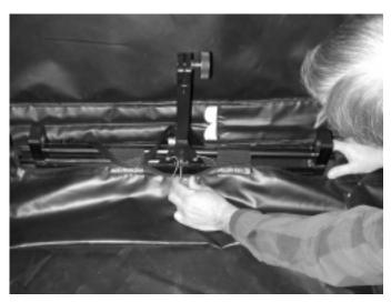
4. Raise both stanchions and pull frame out unit it is fully extended. In both stanchions for both frames, insert/inch pin into bottom hole to lock frames in place.
