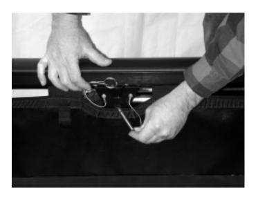
9. Repeat for the other handle (slide in past locator bushing, slide out till stops, rotate and insert pin).
