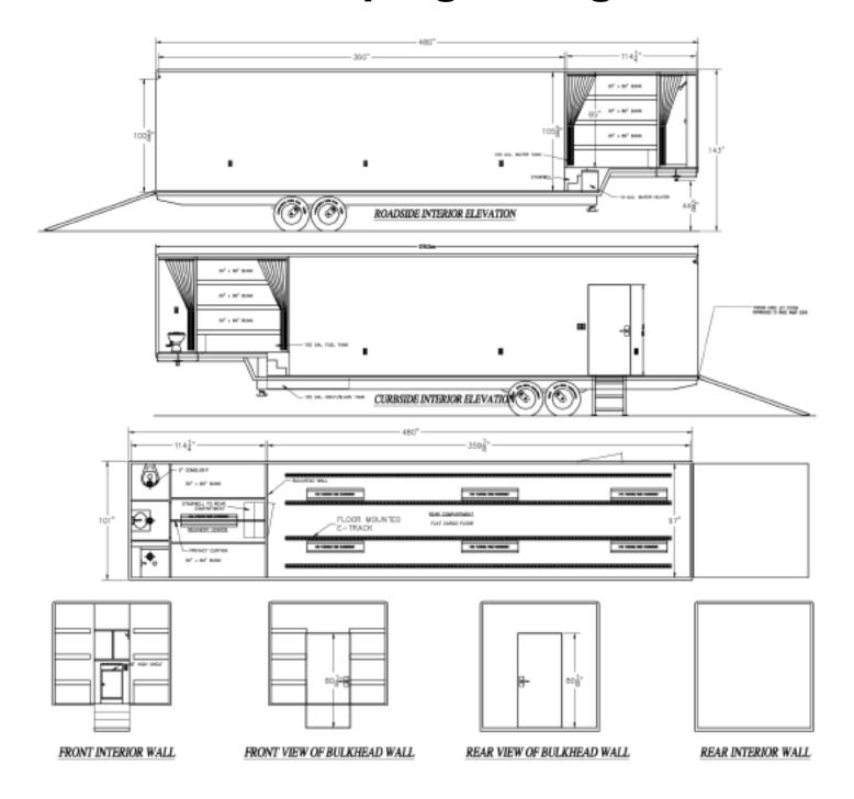
When sleeping-showering-lavatory facilities are necessary, the SR2011 is designed to sleep 6 individuals at a time with a privacy curtain. Hot Water Heater; Fresh Water and Black Water Holding Tanks are built in.
